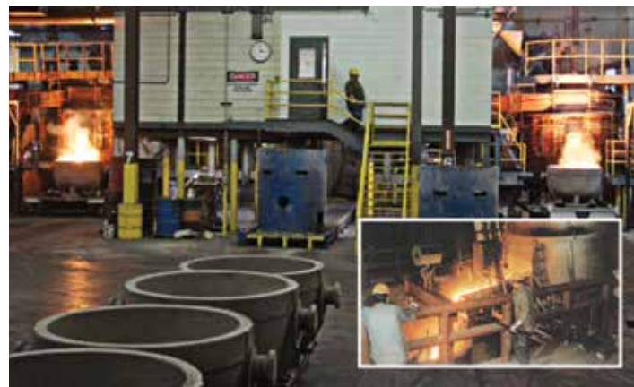
Dual electric arc furnaces double pyrometallurgical processing throughput to help assure maximum recovery of remaining PGMs in spent catalysts—including rhenium.
