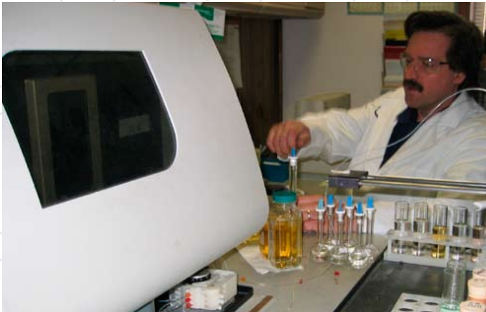
Inductively coupled plasma (ICP) emission spectroscopy for accurate and precise analysis of precious metals samples; our analytical laboratory also uses classic volumetric, gravimetric, fire assay techniques, advanced X-ray fluorescence equipment, and atomic absorption (AA) techniques.
