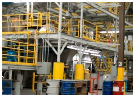
Sabin's automated sampling system captures dust generated during the sampling process for subsequent recovery of precious metals.
