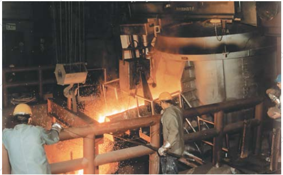
This electric arc furnace represents the latest technology for refining spent PGM catalysts.
