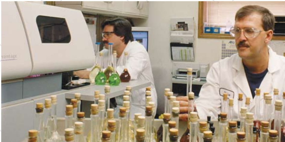
Inductively coupled plasma (ICP) emission spectroscopy helps assure accurate PGM analysis of spent catalysts samples.
