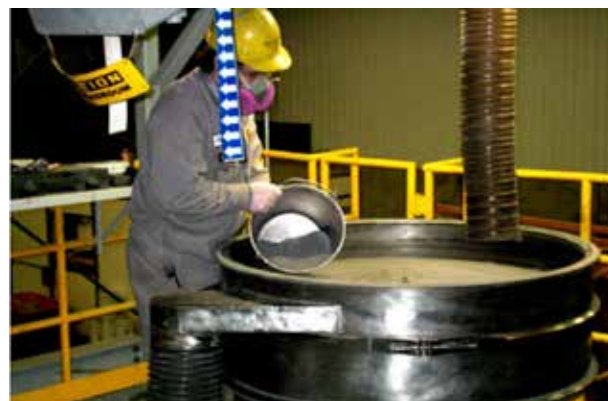
Figure 1. Oversized materials (after re-working) are inspected to assure sample particle sizes under -40 mesh.
