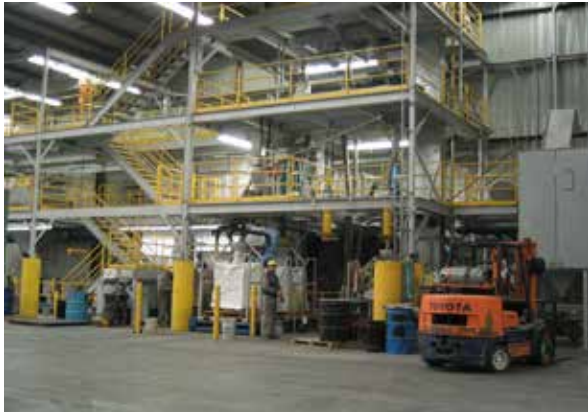
Figure 2 The continuous catalyst sampling system generates homogeneous, consistent, and reproducible intermediate samples. Automated systems produce samples that accurately represent entire lots of spent catalysts. To help assure materials balance accountability, independent dust collection systems (one for the primary sampler and one for the secondary sampler) are employed.
