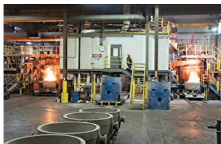
FIG. 2. Electric arc furnaces speed pyrometallurgical processing throughput to assure maximum recovery of remaining PGMs—and rhenium—in spent catalysts.
